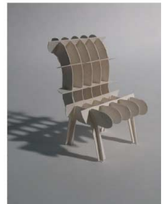
Figure 10. Paper chairs created using the system and cut with a cutter plotter (each chair is about 70 mm in height).
